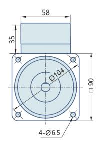
40 Watt : AC Geared Motor With Lead wires
