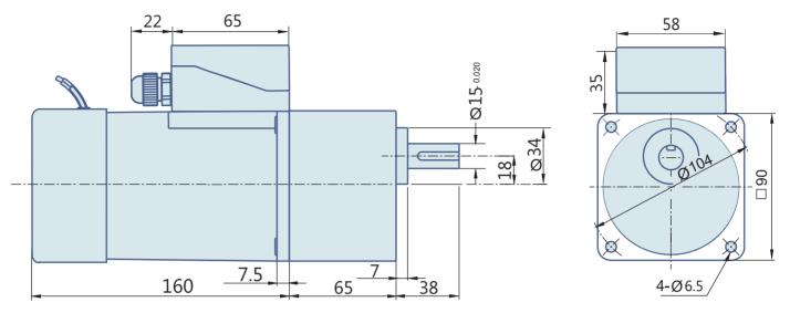
40 Watt : Round AC Induction Motor With Terminal Box
