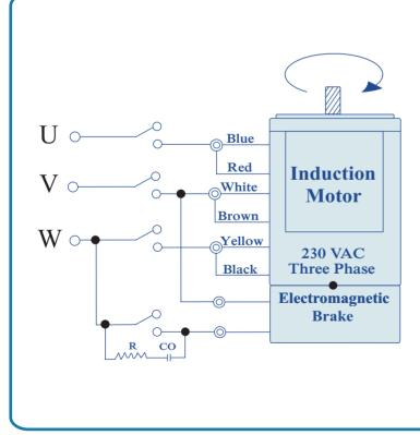
When Sw1 is switched ON, Electromagnetic Brake is released & motor starts rotating. When Sw1 is switched OFF then Electromagnetic Brake will be applied stopping the motor immediately & holding the load.
