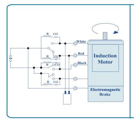
When Sw1 is switched ON, Electromagnetic Brake is released & motor starts rotating. When Sw1 is switched OFF then Electromagnetic Brake will be applied stopping the motor immediately & holding the load.
